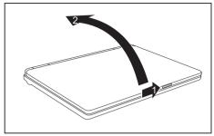
► Slide the release button in direction of the arrow (1) and open the LCD screen (2).
